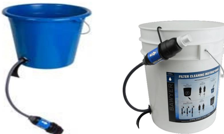
**Sawyer SP 180 water purifier bucket system kit (without bucket): filtering and purifying up to 780 litres of clean water per day with 0.02 micron absolute filtration.** This system has an output of 1 litre per minute when used as a gravity system with a bucket (not included)
